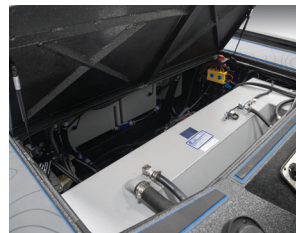
XR21 REAR STORAGE TO ACCESS FUEL TANK AND BATTERIES
