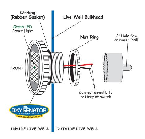
The Oxygenator shuts off automatically when you drain your live well. Although, if unit is connected directly to a battery, green light remains on at all times, but the emitter is not operating. The LED draws insignificant amps. Some manufacturers wire to a switch, some do not.
